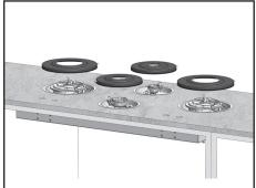
7. Place the heat shields with their sealing rings attached over the burners and secure them using the supplied screws.
