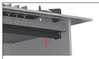
3. Place the beams between the cabinet and position it against the under side of the PITT® cooking unit. ATTENTION: FOR THE POSITIONING, SEE STEP 4.
