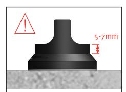
15. **Stop** tightening the set screws when the bottoms of all knobs are inside their sealing scales. The knobs must be within **5-7mm above their scales**.
