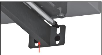
6. Push the beams firmly against the underside of the PITT® cooking unit and tighten the upper two screws completely. Then, tighten the lower screws completely.
