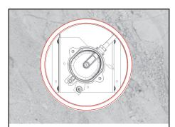
6. Make sure the flanges are concentric inside the cut-outs. WARNING if they are off centre they will not function properly.
