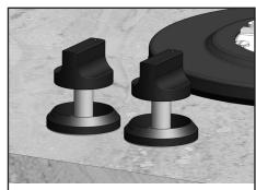
12. Firmly press down the control knobs on the gas tabs with the dots facing forward. Release the knob and make sure it springs back up to its resting position.
