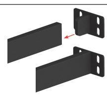
2. Place the inserts into the ends of the beams that have been cut to size.
