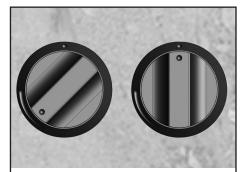
20. Check the knob(s) if they have enough space to push and turn smoothly in the sealing scale. If not remove the sealing scale gently and glue it again.
