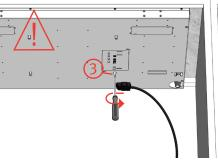
17. Tighten the **centre** set screws (group 3 as shown in step 3) **hand tight**, make sure the **heat conductor** make **full contact** with the **benchtop**.
