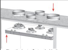
5. Place the heat reflectors inside the cut-outs and gently position the unit beneath the benchtop. Make sure the heat conductor stays in position.
