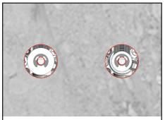
11. Gently shift the unit into a position where all **gas tab pins** are in the **center** of their **cut-outs**.
