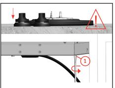
14. Tighten the frontal set screws (group 1 as shown in step 3) by turning them clockwise. This brings the heat conductor up to the benchtop.
