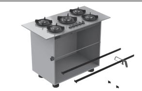
1. Determine the dimensions of the cabinet and cut the support beams with the saw. ATTENTION! Correct length of the beam = the dimension of cabinet on the inside - 4 mm.
