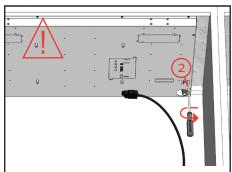
16. Tighten the **rear** set screws (group 2 as shown in step 3) **hand tight**, make sure the **heat conductor** make **full contact** with the **benchtop**.
