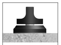
13. After placing the knob there should be a small gap between the bottom of the knob and the top of the sealing scale.
