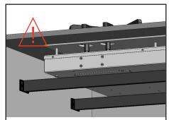
21. Make sure the heat conductor makes full contact with the benchtop and support the **unit** with a **support beam** to lower the tension on the benchtop.
