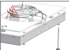
4. Lower all the set screws until they rise just slightly above the unit. When done place the heat conductor on top of the unit.
