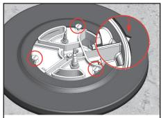
9. Align the cutout in the high burner heat shield(s) with the rib inside the burner(s) and secure it with 3 screws.
