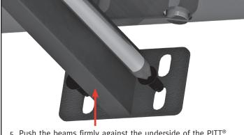
5. Push the beams firmly against the underside of the PITT® cooking unit and tighten the lower two screws by hand. Repeat this step for the other side of the cabinet.
