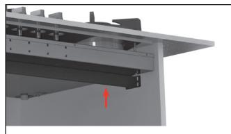
3. Place the beams between the cabinet and position it against the under side of the PITT® cooking unit. ATTENTION: FOR THE POSITIONING, SEE STEP 4.
