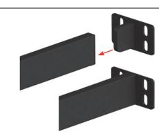
2. Place the inserts into the ends of the beams that have been cut to size.
