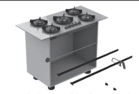
1. Determine the dimensions of the cabinet and cut the support beams with the saw. ATTENTION! Correct length of the beam = the dimension of cabinet on the inside - 4 mm.
