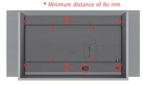
4. Position the beams in such a way that the screws, gas connection and the electricity block are freely accessible.
